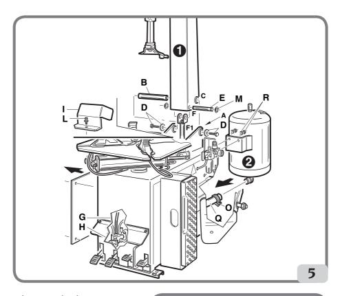
(fig. 5a) until P (fig. 5a) is 3-4mm. - Assemble the column guard I (fig. 5) and lock it with the screws and
