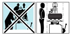
are outside of the vertical cylindrical volume occupied by the wheel. Do not approach.
