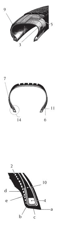
is the outer part of the bead. The base (c) is the area resting against the rim. The groove (d) is the concave part against which the rim shoulder rests.
