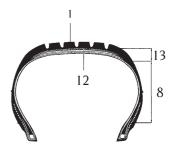
called a belt. The tread and sidewall work with different, independent rigidities, so during rolling, sidewall flexure is not transmitted to the tread.
