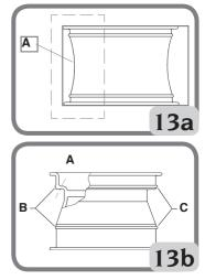
Wheels with pressure sensor - Fig.13C. To work correctly on these wheels and avoid damaging the sensor (which can be incorporated in the valve, secured to the belt, glued inside the tyre, etc.) suitable mounting/demounting procedures must be observed (refer to "Approved mounting/demounting procedure for runflat and UHP tyres").
